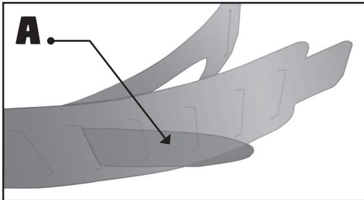
**A:** Bring the ends of the strap together by curving them away from the face shield to form a band. Insert the "Strap Lock" into the desired "Strap Lock Slot" as pictured above.
