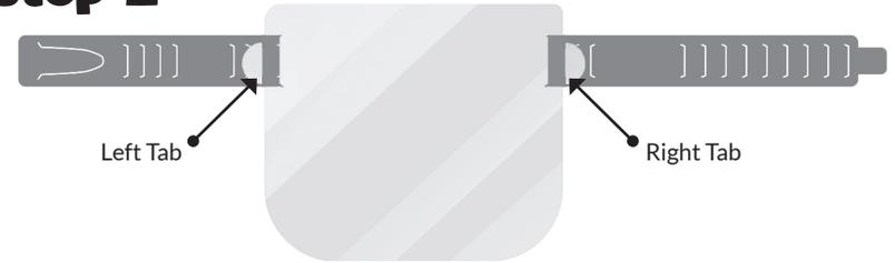
Insert the tabs on the side of the face shield into the "Shield Tab Slots" on the strap as pictured above. Choose the slots that fit the child's face best.
